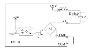
Fig 4-13 Wiring method 1 of multi-function output terminal Y1
