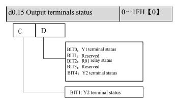
Fig.6-49 Output terminal status
