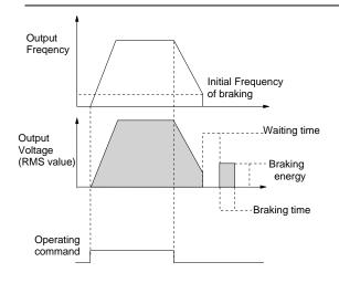
Fig.6-5 Dec-to-stop + DC injection braking
