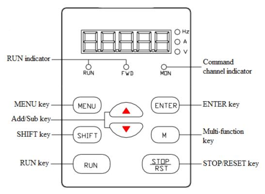
Fig.5-1 Illustration of operation panel
