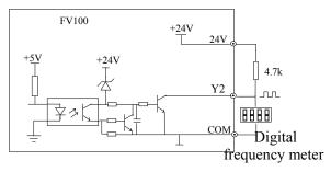
Fig 4-15 Wiring method 1 of output terminal Y2
