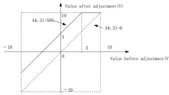
Fig.6-32 The relationship curve between analog output and zero offset
