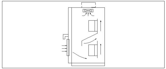
Fig 3-3 Installation of several VFD
