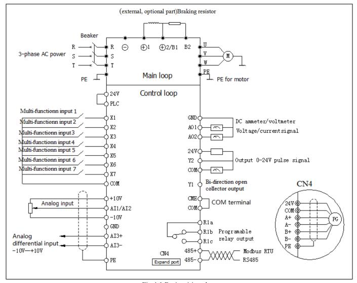
Fig.4-1 Basic wiring chart
