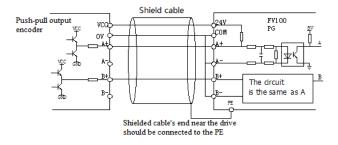
Fig.4-19 Wiring of push-pull output encoder
