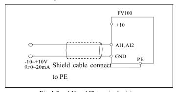
Fig 4-3 AI1, AI2 terminal wiring
