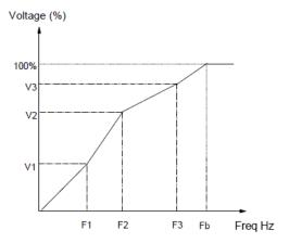
V1~V3: Voltage of sections 1~3 F1~F3: Freq of sections 1~3
