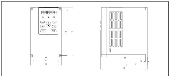
Fig 2-2 FV100-5T-0037G/0055L and lower power VFD
