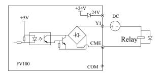
Fig 4-14 Wiring method 2 of multi-function output terminal Y1
