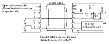
Fig.4-18 Wiring of open collector output encoder
