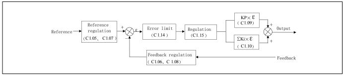
Fig.6-41 Principle diagram of process close-loop control
