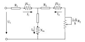
Fig. 6-33 Motor's equivalent circuit In Fig. 6-33, R1, X11, R2, X21, Xm and I0 represent stator's resistance, stator's leakage inductance, rotor's resistance, rotor's leakage inductance, exciting inductance and current without load respectively. The
