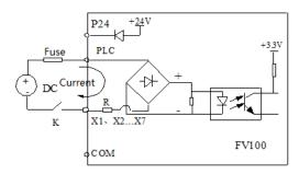
Fig.4-8 Wiring of external power supply
