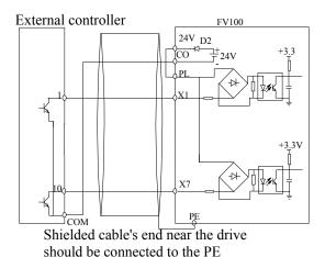
Fig.4-9 Use internal power supply for Source connection
