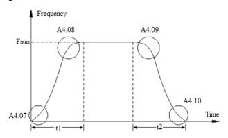
Fig.6-14 Acc/Dec starting time and ending time
