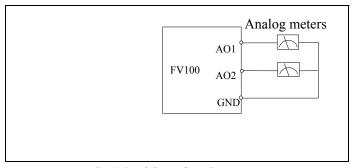
Fig.4-6 Wiring of analog output
