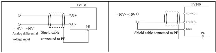
Fig 4-4 AI+, AI- differential voltage input wiring
