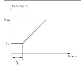
Fig.6-3 Starting frequency and starting time
