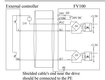
Fig 4-12 Use external power supply for drain connection
