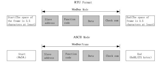
Fig.10-2 Modbus protocol format
