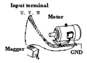
Fig. 1-1 checking the insulation of motor
