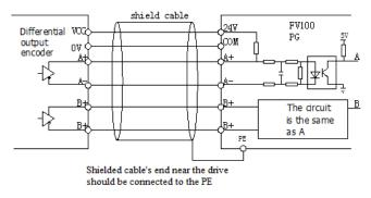
Fig 4-17 Wiring of differential output encoder
