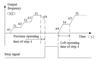
Fig.6-50 Start mode 1 of PLC function
