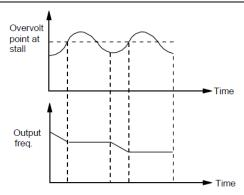
Fig.6-39 Over-voltage at stall
