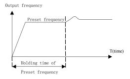
Fig.6-45 Preset frequency of close-loop operation
