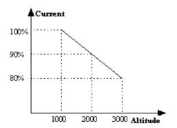
Fig. 1-3 Derating Drive's output current with altitude
