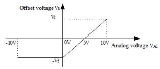
Fig.6-38 Offset of output voltage The output voltage corresponding to the setting frequency in the V/F curve is V/F, then the relationship between analog input and offset voltage is as follows: If analog input VAI is -10V $\sim$ 0V or 4mA, then the corresponding offset voltage is –V or F. If analog input VAI is 10V or 20mA, then the corresponding offset voltage is V or F.
