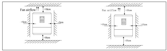
Fig 3-1 Installation interval (Power below 45kW)
