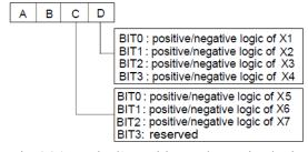
Fig.6-24 terminal's positive and negative logic
