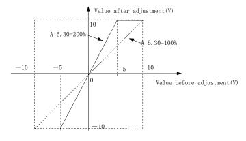
Fig.6-31 Relationship curve between analog output and gain
