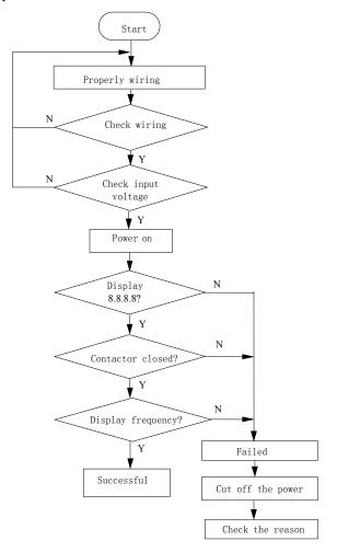
Fig.5-5 Procedures of first-time start-up
