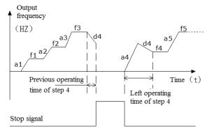
Fig.6-51 Start mode 2 of PLC function Hundred's place of LED: Save after power off 0: Not save
