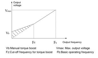
Fig.6-2 Torque boost(shadow area is the boostedvalue)
