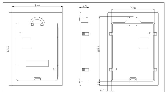
Fig 2-5 Installation box dimension
