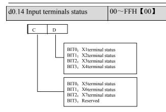
Fig.6-48 Input terminals status This parameter is used to display the status of  $X1\sim X7$ . 0 indicates OFF status,1 indicates ON status.
