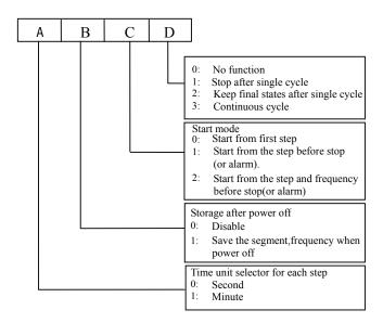
The unit's place of LED: PLC function running mode 0: No function.
