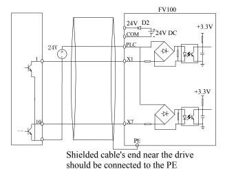
Fig 4-11 Use external power supply for source connection
