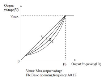
Fig.6-35 Torque-reducing curve
