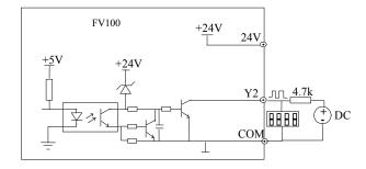
Fig.4-16 Wiring method 2 of output terminal Y2
