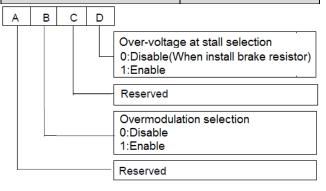
During deceleration, the motor's decelerate rate may be lower than that of drive's output frequency due to the load inertia. At this time, the motor will feed the energy back to the drive, resulting in the voltage rise on the drive's DC bus. If no measures taken, the drive will trip due to over voltage.
