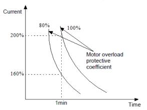
Fig.6-34 Motor's overload protection coefficient
