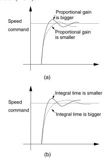
Fig.6-14 The relationship between step response and PI parameters of speed regulator(ASR)
